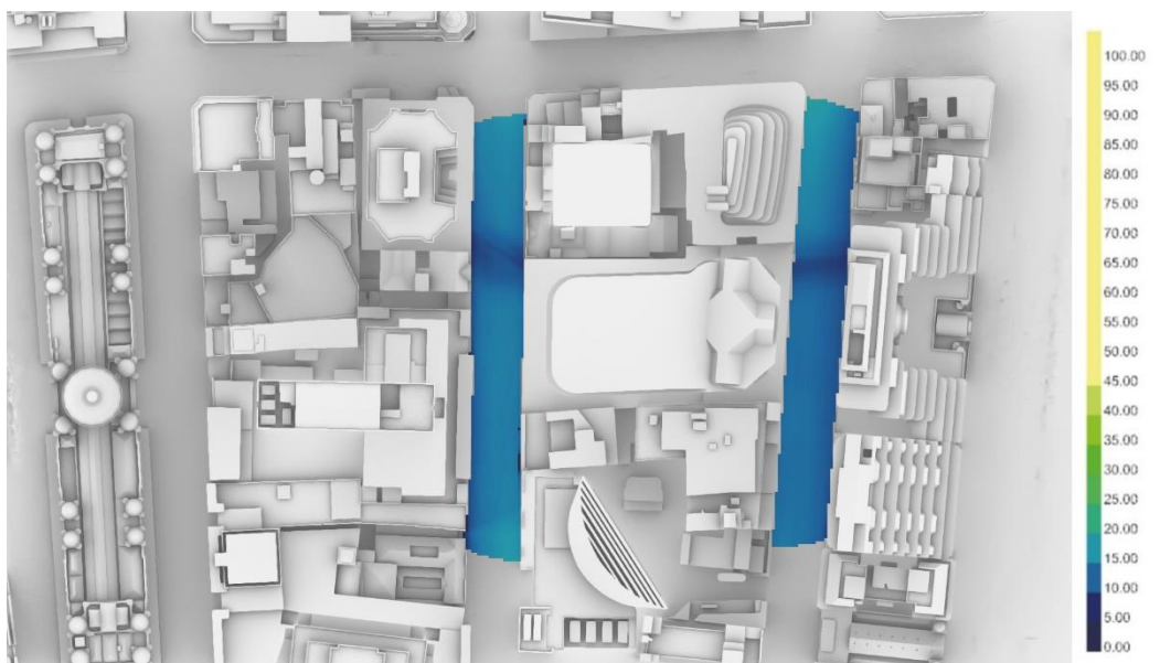
Figure 4.2a Sky View Factor for base case envelope.
